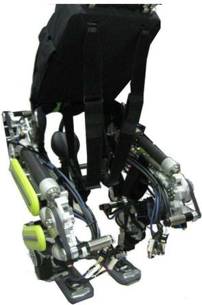
The lower-body strength-augmenting exoskeleton "XO"
