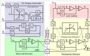
Integrated model of control, electronics, and mechanisms
