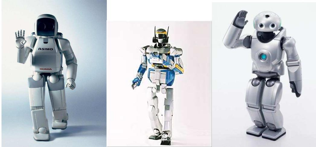
Figure 1.1: **Examples of stiffly-actuated, position-controlled humanoid robots.** *Left:* The humanoid robot “Asimo”, developed by the Honda Motor Corp. *Middle:* HRP-2, developed by Kawada Industries, Inc. together with Humanoid Research Group of National Institute of Advanced Industrial Science and Technology (AIST), Japan. *Right:* QRIO, developed by Sony Corp.
