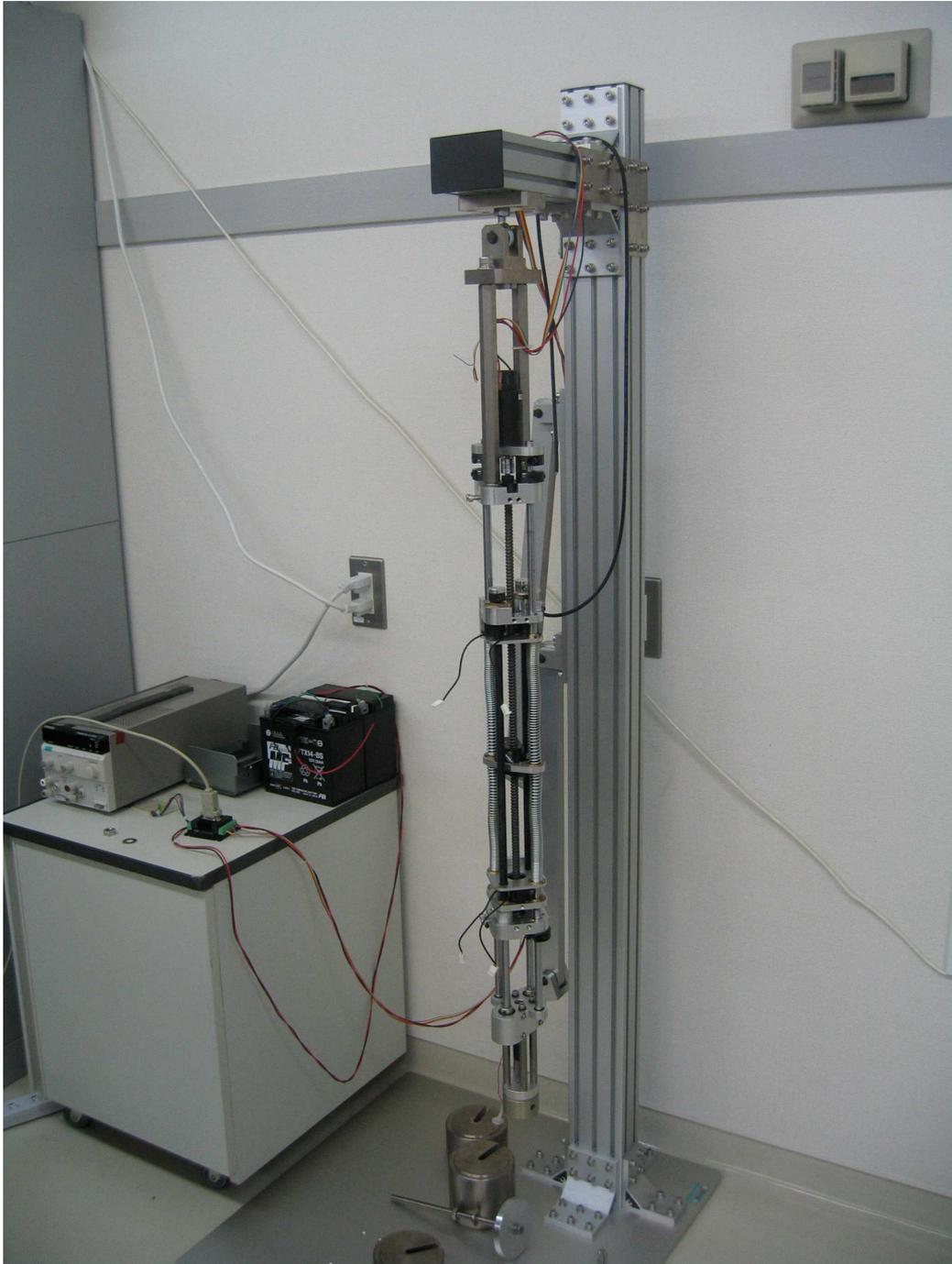
Figure 4.4: **Photos of the VSSEA.** *Left:* The VSSEA on a table. Extra sensors have been fitted to the VSSEA for testing. *Right:* The VSSEA in a vertical-hang test configuration. Two other configurations are possible: horizontal and “hopping” modes.
